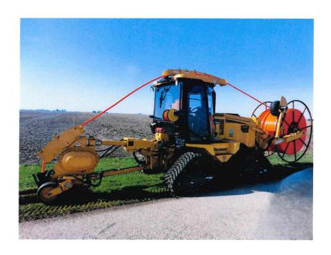
This boring machine is being used to install fiber optic lines underground.
